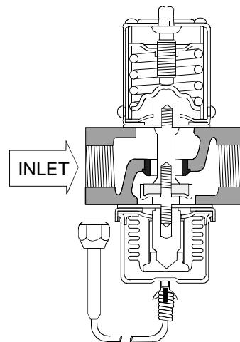
**Figure 3: Threaded Type Reverse-Acting Valve Cross Section**
