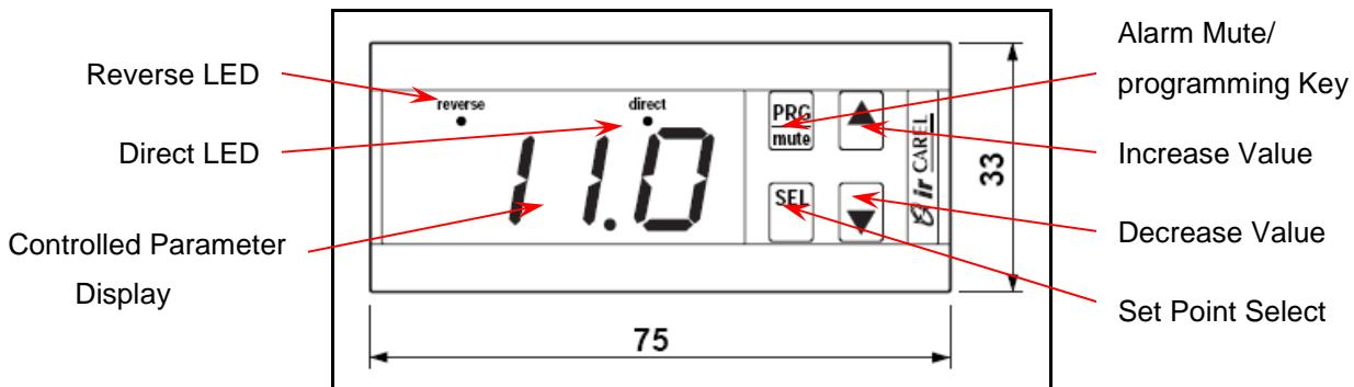
Figure 7    IR 32 Controllers
