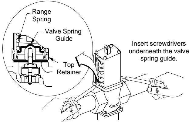
Figure 6: Manual Flushing
