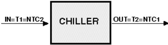
If  $NTC1=T1$ , the set-point will be 'NTC1-NTC2', that is 'T1-T2' which has to be +5°C ( $St1=+5^{\circ}C$ ). The 'Reverse' control action will be applied ( $C0=2$ ) as the controller has to energize outputs as the 'T1-T2' difference decreases (towards 0). If you set differential=2°C ( $P1=2$ ), high temperature threshold=40°C ( $P26=40$ ) and a 30 minutes' time-delay ( $P28=30$ ), the operating mode will be as illustrated in the graph below:
