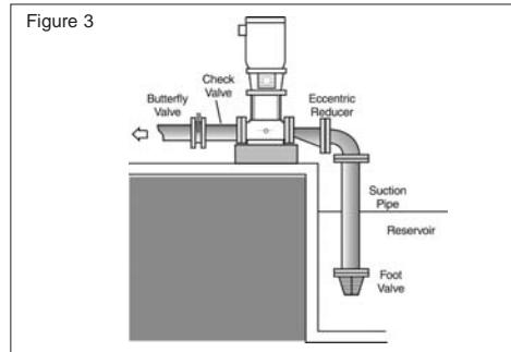
\* CRN-SF pumps cannot be used for suction lift. The suction pipe should have a fitting on it for priming.
