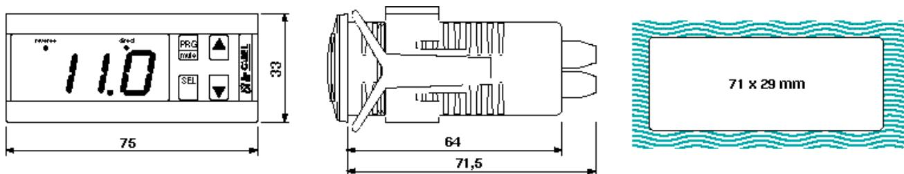
***IR32 - Panel mounting*****IRDR - montaggio da guida DIN**
