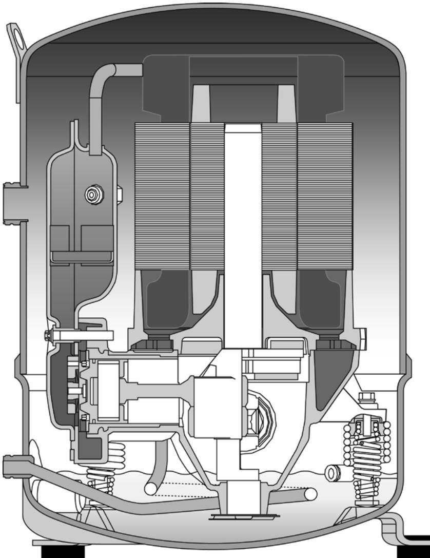
The compressor design allows for the motor to be 100% suction-gas cooled.
