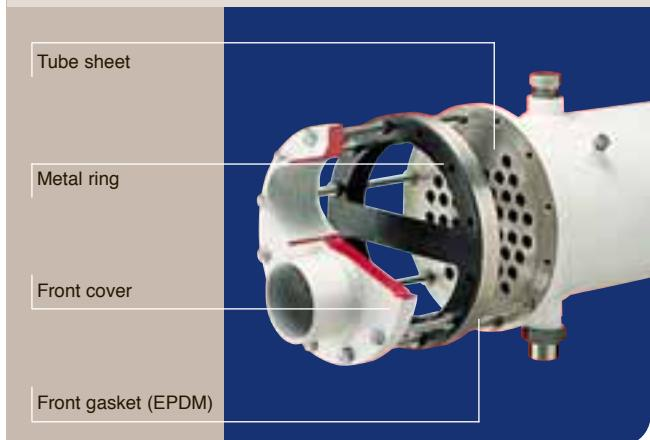
CDEW series of shell and tube condensers has been optimised by Alfa Laval's R&D dept. and Laboratory in order to ensure the highest performance with HFC-R407C. This refrigerant is particularly affected by glide and this phenomenon can be relevant during the condensing phase causing losses in performance if standard condensers designed to operate with azeotropic refrigerant are used. Thanks to its special design and sizing, CDEW condensers can now reduce 3K
