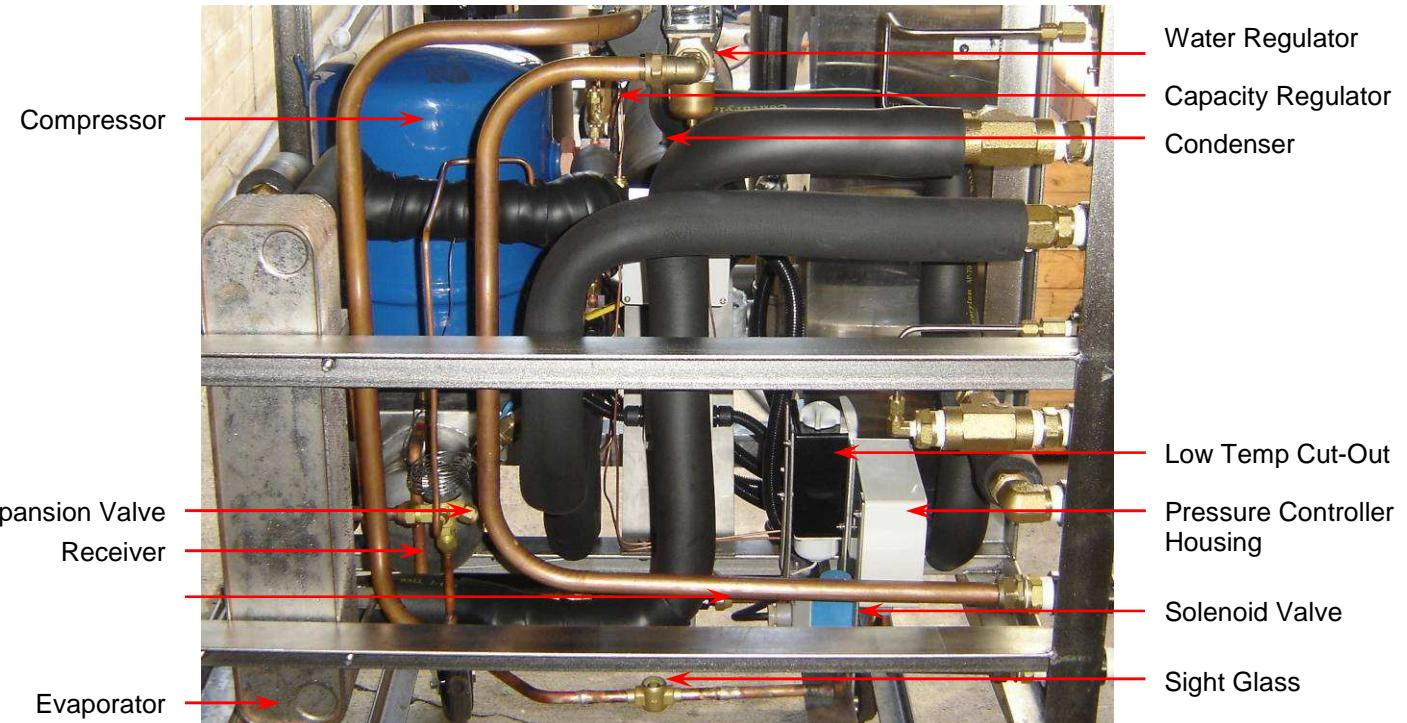
**Figure 6      Refrigeration Circuit**
