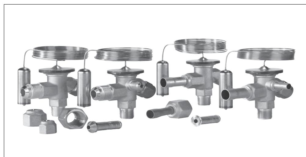
Thermostatic expansion valves regulate the injection of refrigerant liquid into evaporators. Injection is controlled by the refrigerant superheat. Therefore the valves are especially suitable for
