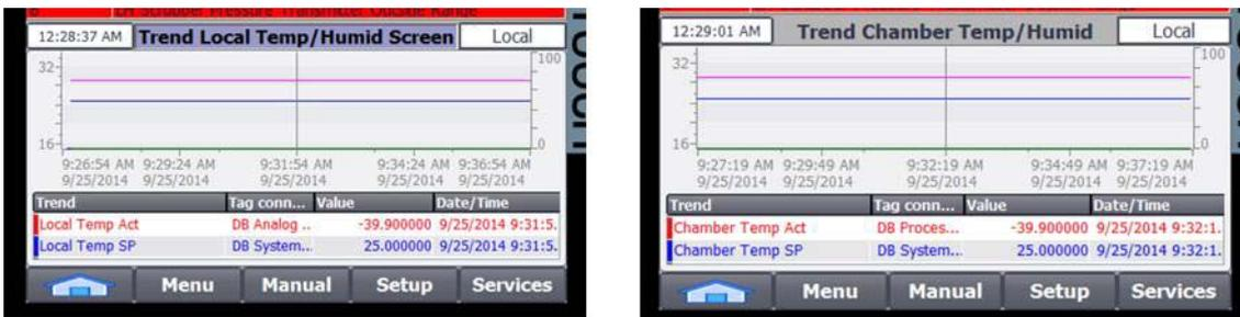
Fig 5.11 Temperature & Humidity Trend Screens
