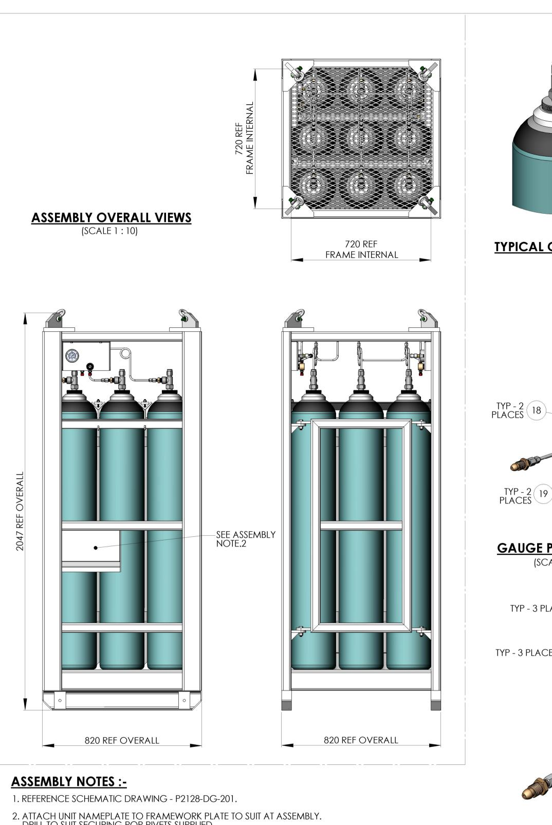
ATTACH UNIT NAMEPLATE TO FRAMEWORK PLATE TO SUIT AT ASSEMBLY. DRILL TO SUIT SECURING POP RIVETS SUPPLIED.
