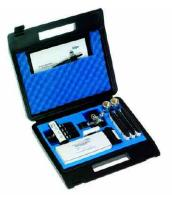
The Bauer Aerotest Simultan HP allows reliable measuring of CO,  $CO_2$ ,  $H_2O$  and oil and also detects synthetic oils. It can be used on the compressor or directly on the cylinder and allows quick check on site. The measuring of breaking air is in accordance with DIN EN 12021.
