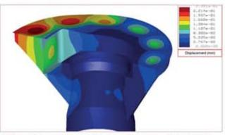
FIGURE 1. Displacement magnitude fringe plots under external pressure due to 55 msw (0.558 MPa): view at x350 magnification
