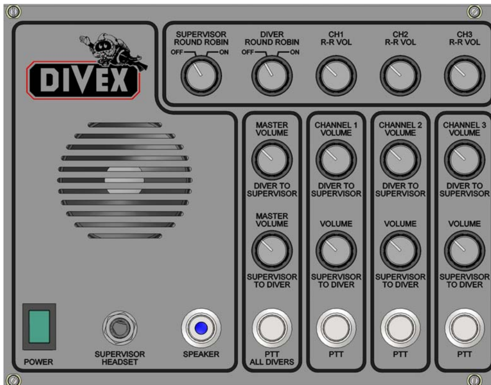
Fig 3.2 Power & Audio Control Switches
