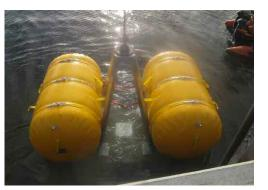
Totally Enclosed Lifting Bags in situations where insufficient depth of water precludes the deployment of parachute type lifting bags above the object to be raised, an effective alternative is the use of a cylindrical totally enclosed lifting bag. They can be secured closely to the article or shackled to straps passed underneath it.
