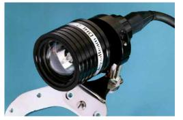
The Aquabeam Diver's Helmet Light, DHL-2 is a hard anodised and marine sealed, aluminium luminaire, offering a variety of build options, beam angles and colour temperatures. In its standard form, it weighs 500 grams dry and 185 grams immersed. Its maximum diameter is 60mm and overall length excluding connector, 101mm. The maximum operating depth of the DHL-2 is 700 metres. All components are available as spare parts.
