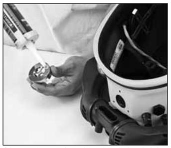
Silicone sealant is used to seal the exhaust body to the helmet shell.
