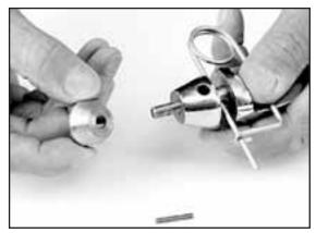
Once the pin is driven out, you can remove the knob from the shaft.
