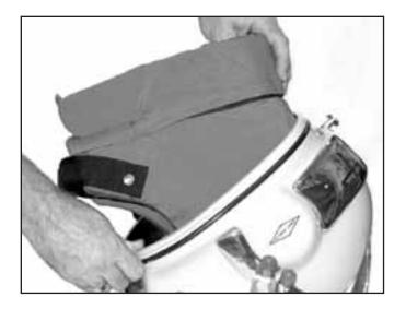
To gain access to the earphones, you must first remove the head cushion.
