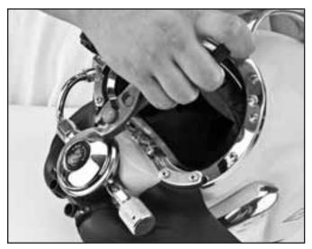
Loosen the nose block knob with a pair of pliers.
