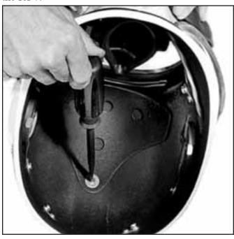
To remove the handle, you must also remove the internal screw.
