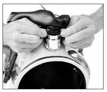
Attach the whisker to the double exhaust main body.
