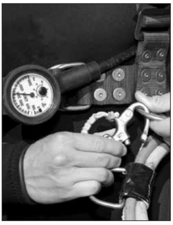
The umbilical must be properly attached to the diver's harness.
