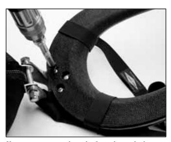
You must separate the yoke from the neck clamp to replace the neck dam.
