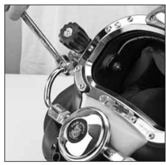
Loosening the bent tube from the side block.
