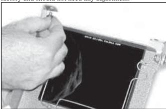
The screws that secure the weld shield insert as shown here.
