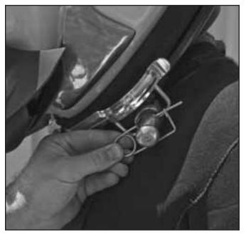
The safety pin must be installed prior to every dive.
