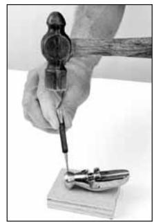
The pin secures the knob on the end of the shaft.
