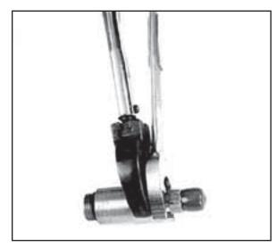
Tighten to 150 inch lbs. (17 Newton Meters) with a torque wrench.
