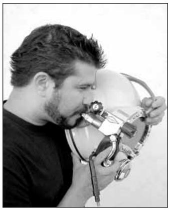
You can test the one-way valve either by attempting to suck air through the valve with the steady-flow valve open, or by connecting the bail-out to the main supply (with the steady flow and regulator adjustment closed) and opening the emergency valve to check for back-flow.
