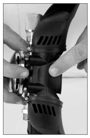
Note the correct alignment of the mold line that spans the whiskers and the exhaust main body.
