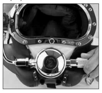
Make sure that the regulator adjustment knob is screwed in and the steady-flow valve is closed before opening the air supply to the helmet.
