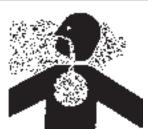
Use silicone sealant in a well ventilated area. Do not breathe the fumes from uncured silicone sealant. These fumes are dangerous and can cause unconscious-
