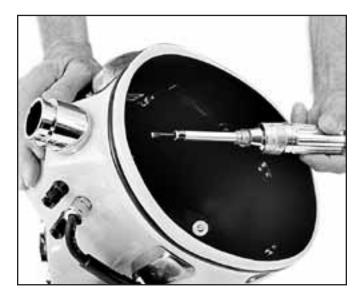
Be sure to install the screws which help to secure the double exhaust body to the helmet shell.
