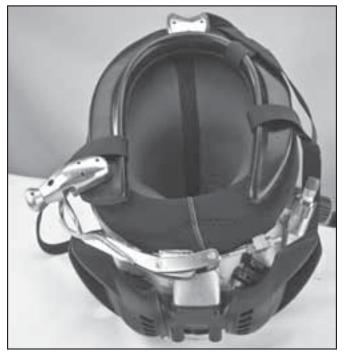
Note the proper engagement of the latch catch mechanism in the top photo on this side of the page. Also note that the centerline of the yoke bisects the entire helmet.
