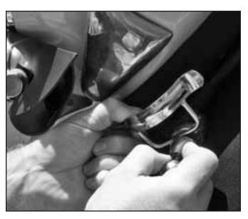
The pull pin must properly engage the bail on the neck clamp.
