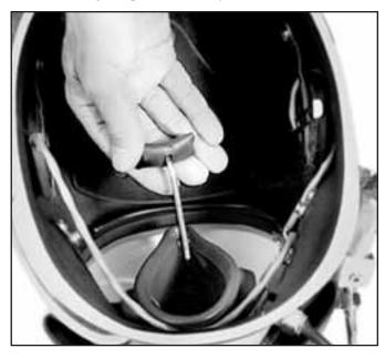
The shaft for the nose block device slides through the hole in the oral nasal mask.
