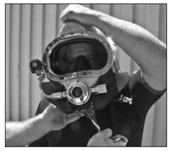
The diver must hold the helmet down while the clamp is swung to their right to fully engage it against the bottom of the helmet. Note how the tender is supporting the clamp mechanism with their left hand.
