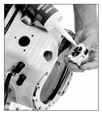
The double exhaust body must be sealed to the helmet shell with RTV.
