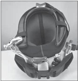
Note that the latch catch mechanism on this side of the page does not properly engage the bail on the neck clamp. Also note the yoke is "skewed" and is not centered across the rest of the helmet.
