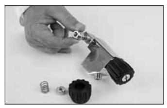
*Installing the packing nut on the valve stem.*
