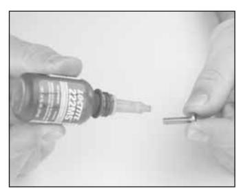
The latch catch assembly must be fastened to the yoke using Loctite® to secure the screws.
