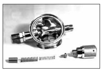
Components to the regulator adjustment assembly.
