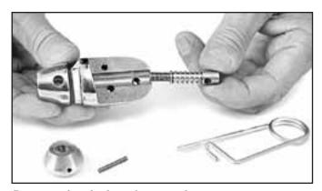
Remove the shaft and spring for service.
