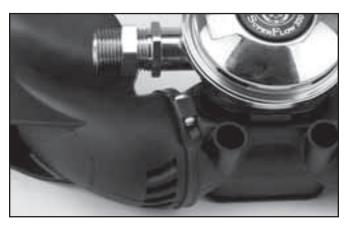
To allow access to the two exhaust valves in the whisker wings, you must first remove the two whisker clamps that hold the whiskers on the exhaust main body. This is the starboard clamp.
