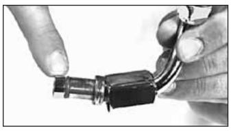
Replace the O-ring on the bent tube if it is worn or damaged.
