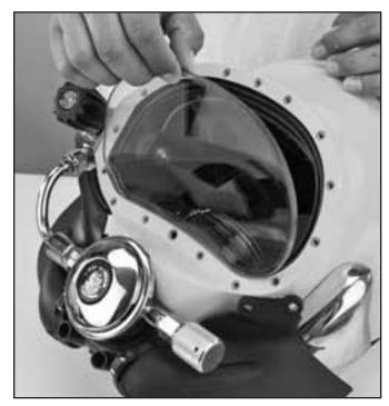
Replace the face port if it becomes badly scratched or shows any signs of damage due to contact with chemicals.
