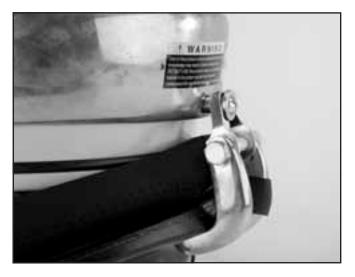
The rear hinge tab must engage the alignment sleeve.
