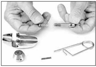
Inspect the spring and shaft and clean in a mild solution of white vinegar.
