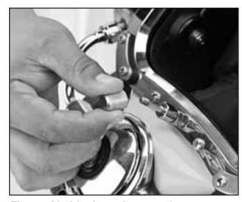
The nose block knob must be removed prior to removing the packing nut.
