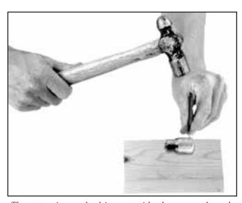
The cotter pin must be driven out with a hammer and punch.
