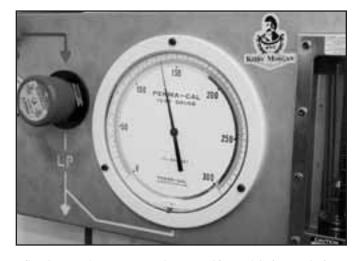
Set the supply pressure to between 135 and 150 p.s.i. before adjusting the regulator.
