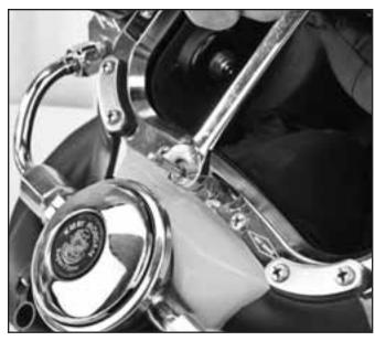
The nose block packing nut must be tightened enough to seal the nose block device shaft but loose enough for the device to slide in and out.
