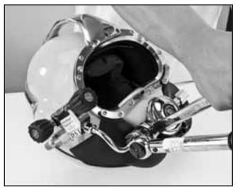
The jam nut and bent tube must be tightened to the proper torque specification.
