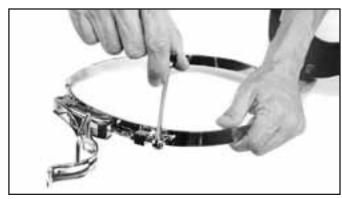
The neck clamp must be periodically inspected for signs of wear and tested for proper closure.
