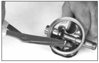
Trim any excess exhaust valve tail from the interior of the regulator.
