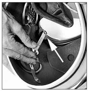
You must remove the nut that secures the air train before you can proceed in removing the side block.
