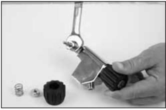
Undo the packing nut.
