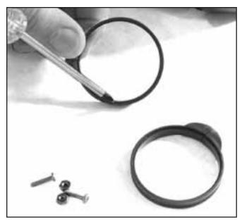
Note the step on the inside of the whisker clamps. These must be oriented in the correct position to retain the whisker wings properly.
