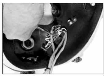
If you are using the terminal block, this is where you will disconnect the earphones from the helmet.
