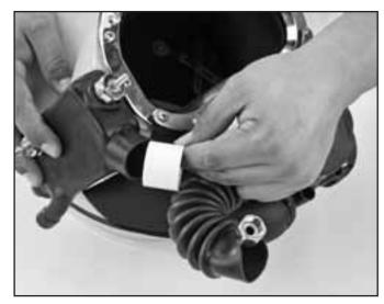
*Install the bent tube at the side block.*
