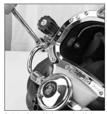
Begin installation of the hot water shroud by loosening the bent tube at the sideblock.
