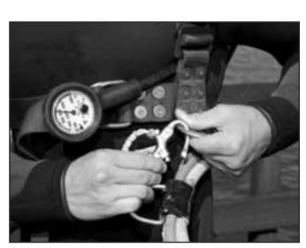
The umbilical should always be attached to the harness to avoid a direct pull on the diver's helmet.
