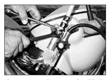
Always use two wrenches to connect the umbilical to the adapter. Use the correct size wrenches whenever possible to avoid damage to the fittings.
