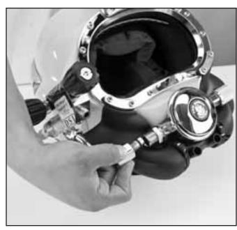
Remove the bent tube assembly before removing the side block.
