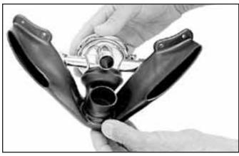
Mount the double exhaust system on the regulator.
