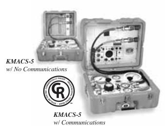
The **Kirby Morgan Air Control System-5 (KMACS)** is a lightweight, portable control box for use in surface supplied air diving operations. The KMACS-5 controls the diver's air supply, communications and monitors the diver's depth. It allows two divers clear push-to-talk (two wire) or round robin (four wire) communications. The KMACS-5 is also available
