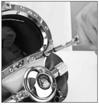
The whiskers must be removed prior to removing the port retainer and port.
