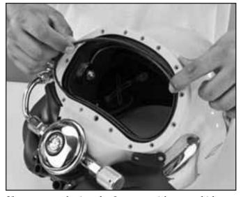
If you are replacing the face port, it's a good idea to replace the o-ring that seals it.
