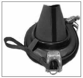
This is how the guide strap should look when it is properly installed (note that yoke/neck clamp is upside down to allow you to see where the strap installs).
