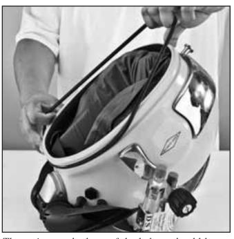
The o-ring on the base of the helmet should be replaced whenever it shows signs of wear.
