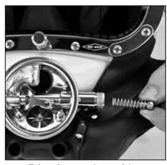
Shake out the spacer, spring set, and piston.
