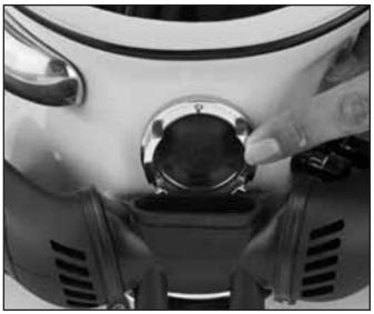
The Quad-Valve<sup>TM</sup> cover must be removed to inspect the water dump valve.
