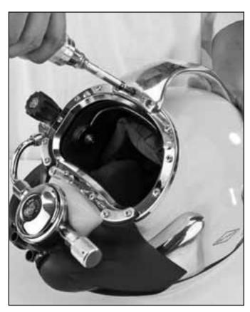
Use a torque screwdriver to tighten the front handle screws to 12 inch pounds.
