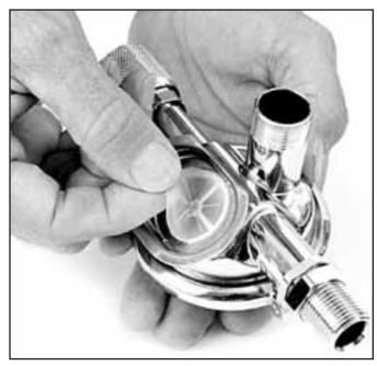
The exhaust valve must make proper contact with the spokes on the exhaust flange. If the spokes are not in proper alignment with each other, the regulator will leak.
