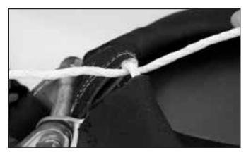
Tie a square knot in the drawstring to secure the dam around the clamp.
