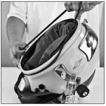
The o-ring on the base of the helmet must be in good condition.
