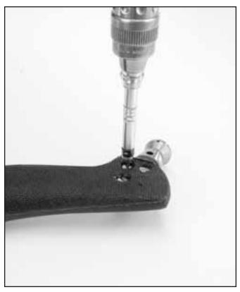
Begin the disassembly of the yoke by removing the latch catch assembly.
