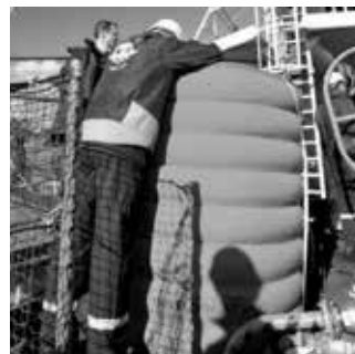
JFD's Inflatable Freeboard Extender - trials on RUBIS Class Submarine
