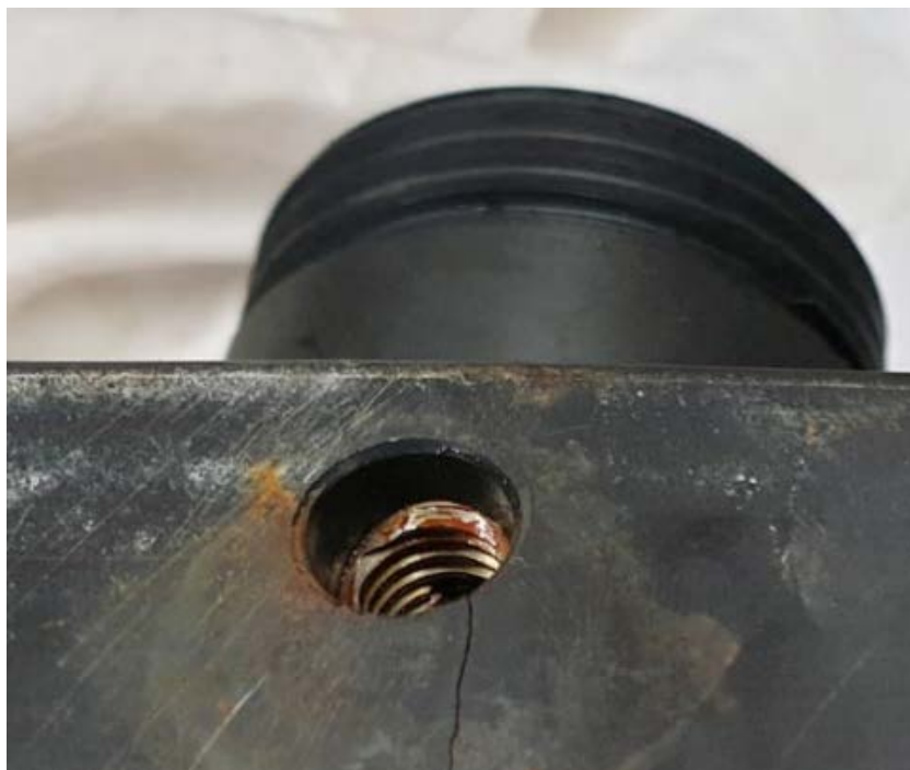
Figure 1 - Cracking at insert pocket
