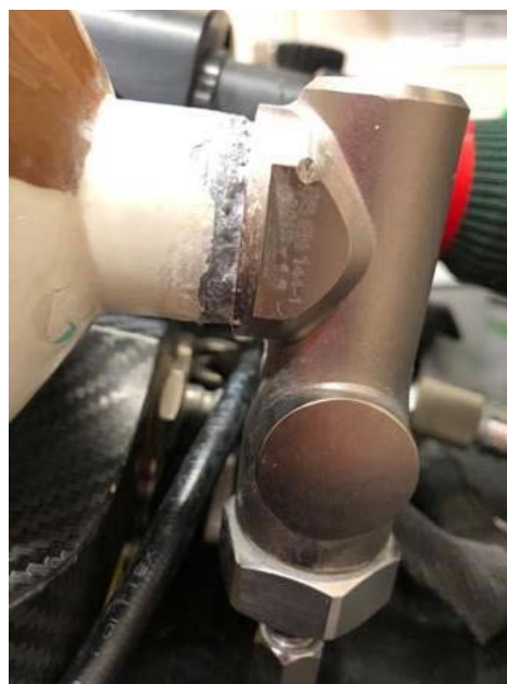
Figure 2 - Excessive Corrosion at Cylinder Neck
