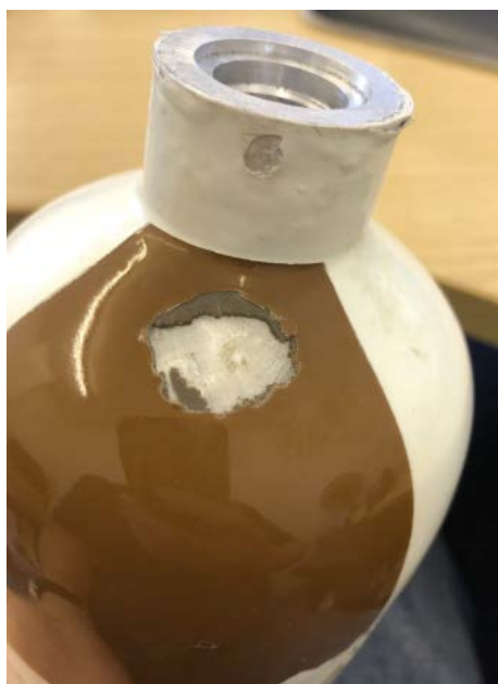
Figure 1 - Flaking External Lacquer
