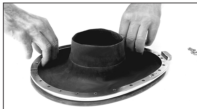
Center the split rings by pressing on the dam and feeling the inside edge of the stepped ring and the split rings.
