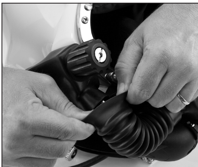
Pull the corrugated tube over the PVC flange at the sideblock.
