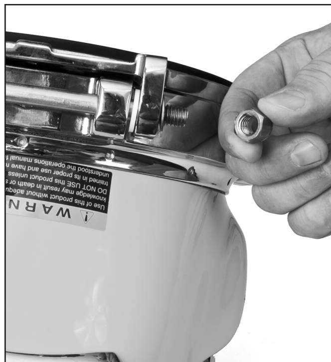
The nut can be started by hand but must be tightened with a socket and back-up wrench.
