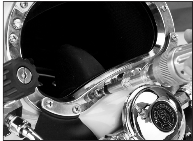
Always use a torque screwdriver to check the tension of the port retainer screws.
