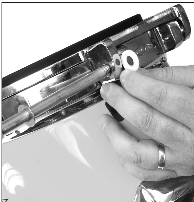
The Teflon® washers are essential to smooth operation of the locking collar.
