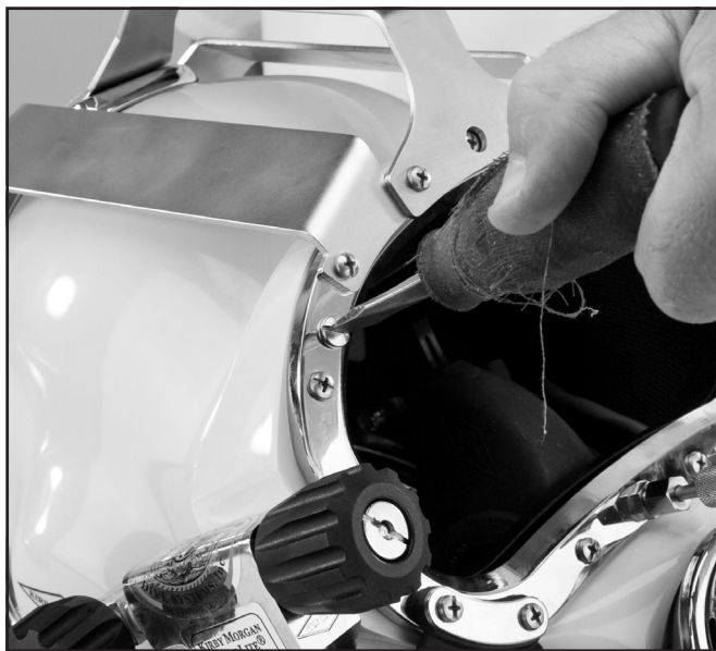
Remove the two plug screws from the port retainer.
