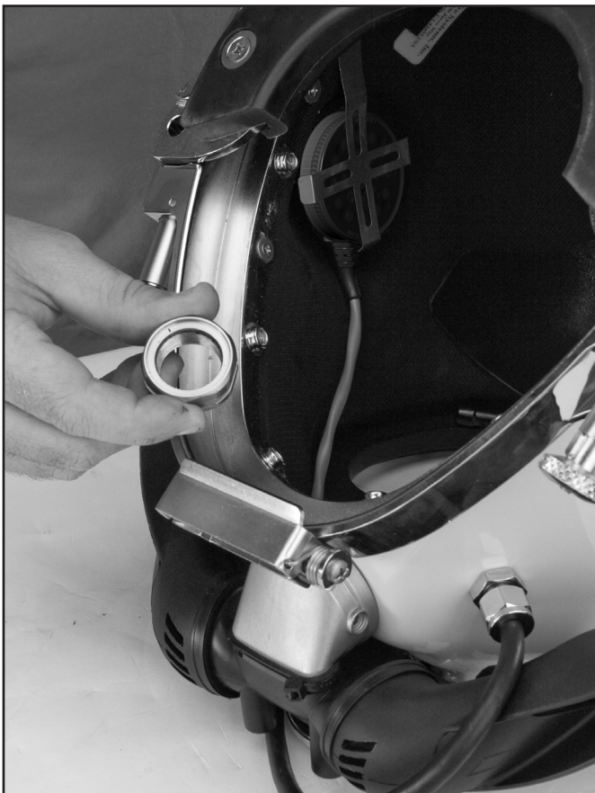
The regulator mount nut must be removed to remove the regulator.
