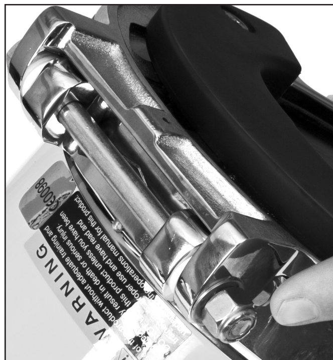
There is no torque value for this nut, but it must be tightened until the bolt is flush with the top edge of the nut.
