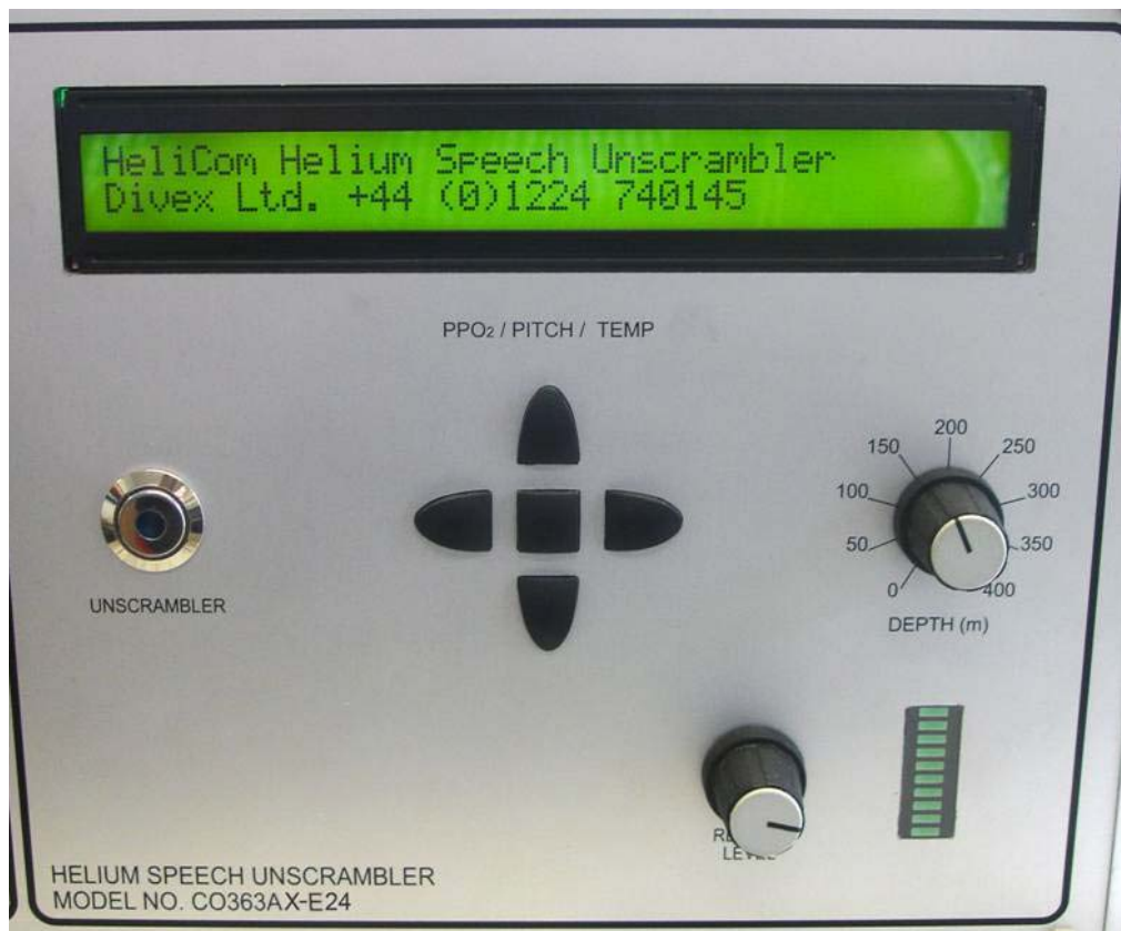
Fig 4.1 User Interface & Keypad
