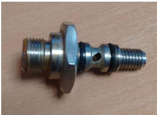
Figure 1 - Damaged Hot Water Spigot
