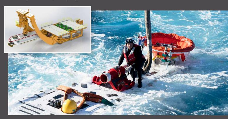
The 3rd generation system has a compact architecture and design. The system can be deployed in multiple layouts; meaning it can also be installed on vessels with unusual deck arrangements. The system is modular and various aspects can be deployed independently – for example individual Deck Decompression Chambers (DDCs) can be deployed independent of the rest of the system for escape support or secondary roles.
