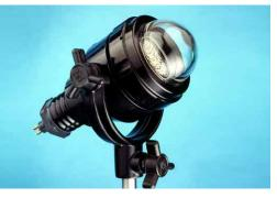
The SFL 3000 (Supersedes MV2000) is a versatile, flood luminaire, designed for operation down to 3000 metres of seawater, SFL 3000 accommodates the range of minican lamps, from 100 to 1,000 watts, operating from 120/240 Vac or 24Vdc.
