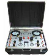
The Divex 2 Diver HP/LP Control Panel is a portable panel, mounted in a robust carry case, incorporating HP and LP air control and depth monitoring for 2 divers.
