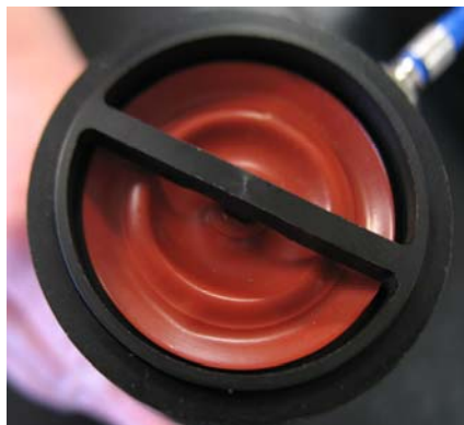
Figure 2: Original Flap Valve during testing
