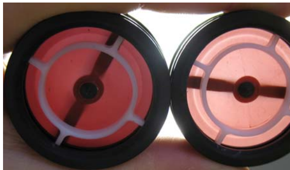
Figure 1: Comparison between original and recent flap valves
