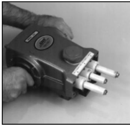
Proper Alignment of Ceramic Plungers for reassembly
