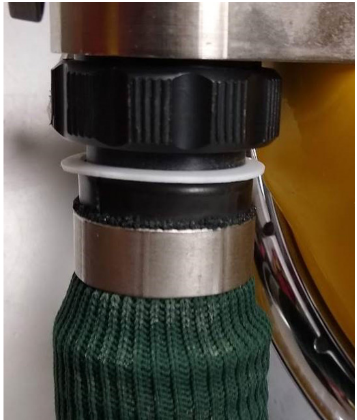
Figure 6 - Helmet Exhale Connection Correctly Made Up (no thread visible)
