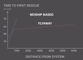
Distance from system to distressed submarine (nautical miles) Flyaway aircraft may need to refuel
