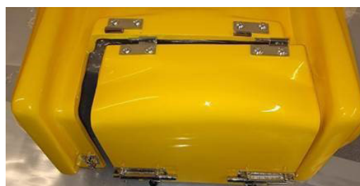
Figure 2 - Incorrect hinges and fitted upside down
