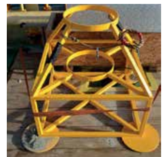
Lightweight, portable Pod Posting Target capable of deployment by ROV
