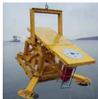
610m rated Pod Posting and Atmosphere Sampling Target for NSRS. Adjustable to 60° subsea.
