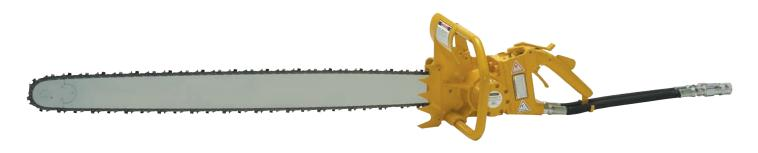
The **CS11** is an extreme duty hydraulic powered chain saw for cutting all types of wood structures underwater - including bridge pilings, pier and dock timbers. It's robust design and high torque gear motor provides divers instant chain speed to cut through the toughest timbers with ease. The power to weight ratio is significantly higher than any other wood cutting chain saw and is available with bar lengths up to 36" (91 cm). Painted hi-visibility yellow.
