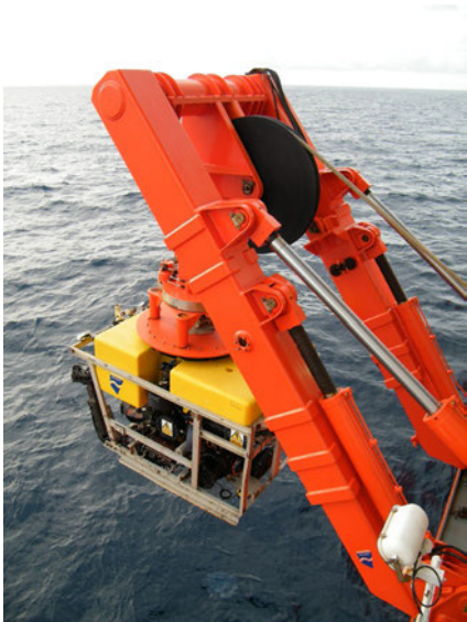
INTERVENTION ROVS Provided by JFD form an integral part of many submarine rescue systems.
